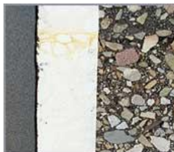
A direct positive reaction in the white substance you can see the brown/yellow colour
